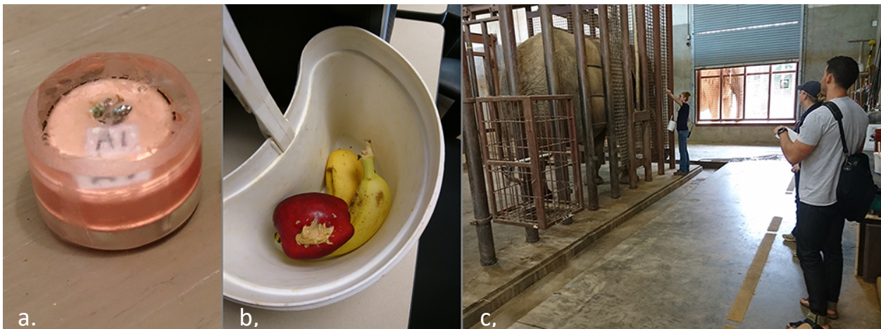
Figure A1. (a) The iButtons (Thermochron DS1921H-F5, Maxim Integrated) were incased within protective epoxy (Loctite Hysol) and labeled to help determine the identity of the consumer (left). (b) We embedded the iButtons within fruits, such as apples, mangoes and bananas (middle). (c) Zookeepers from the North Carolina Zoo fed the baited fruits to individual elephants within their holding pens during one of the regular feeding times.
